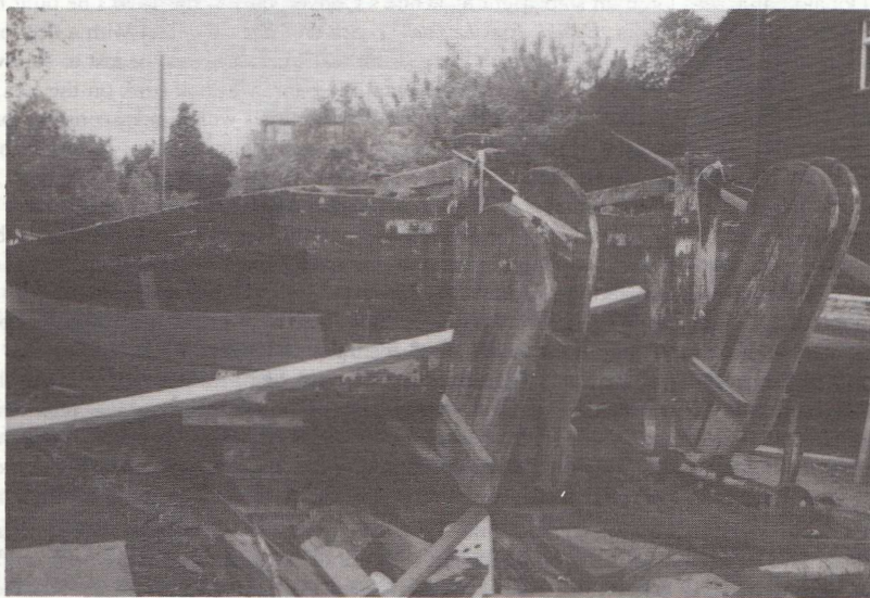
Chelmer and Blackwater Navigation barge Susan out of the water alongside Cook's Yard, Maldon, undergoing substantial rebuilding. Two new planks have been inserted on each side together with new linings and inwales.
